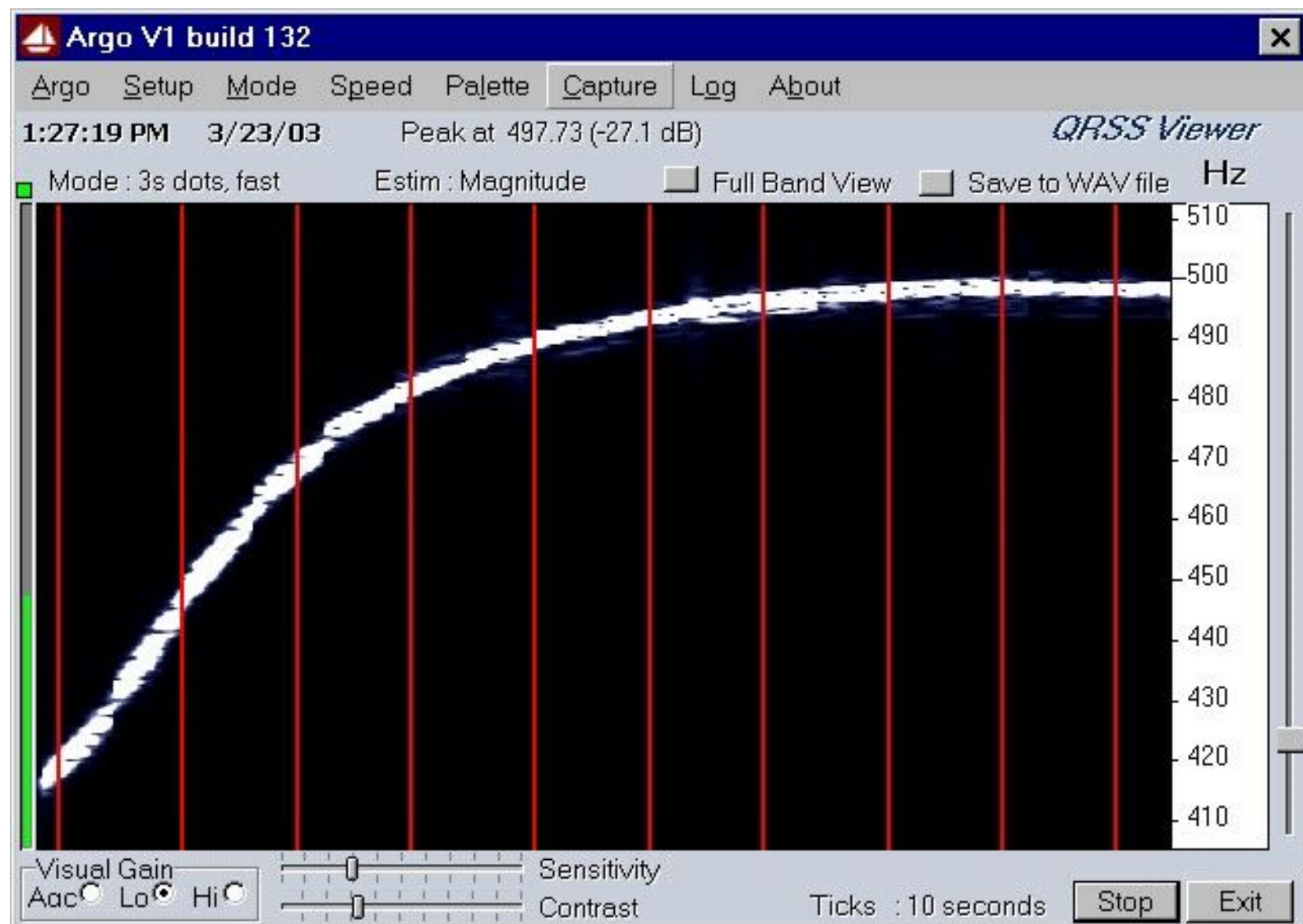
Figure 1 shows the cold start drift over the first 90 seconds of operation. In this case it is about 80 Hz and the absolute error is 2.27 Hz. (0.227 ppm)
