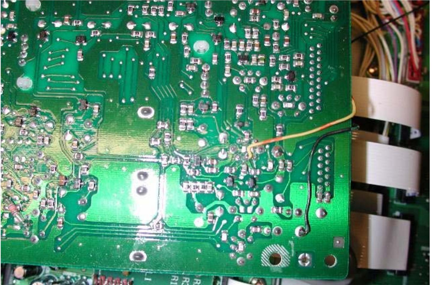
The picture below shows the board back in its normal position. I used glass tape to mount the board on the bundle because I had some. I would have preferred to use some small Velcro tabs or some of the foam sticky tabs, but did not have them on hand. The board is mounted on the cable bundle that runs along the left side of the filter board as viewed from the rear of the radio. This picture was taken so that the front of the radio is at the bottom and the back of the radio is at the top.
