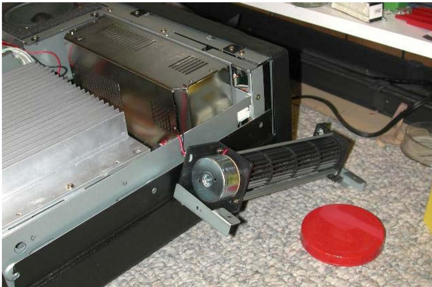
Then you unclip the plastic tabs that hold the cables and remove the heat sink mounting screws and flip up the heat sink to get at the RF board.
