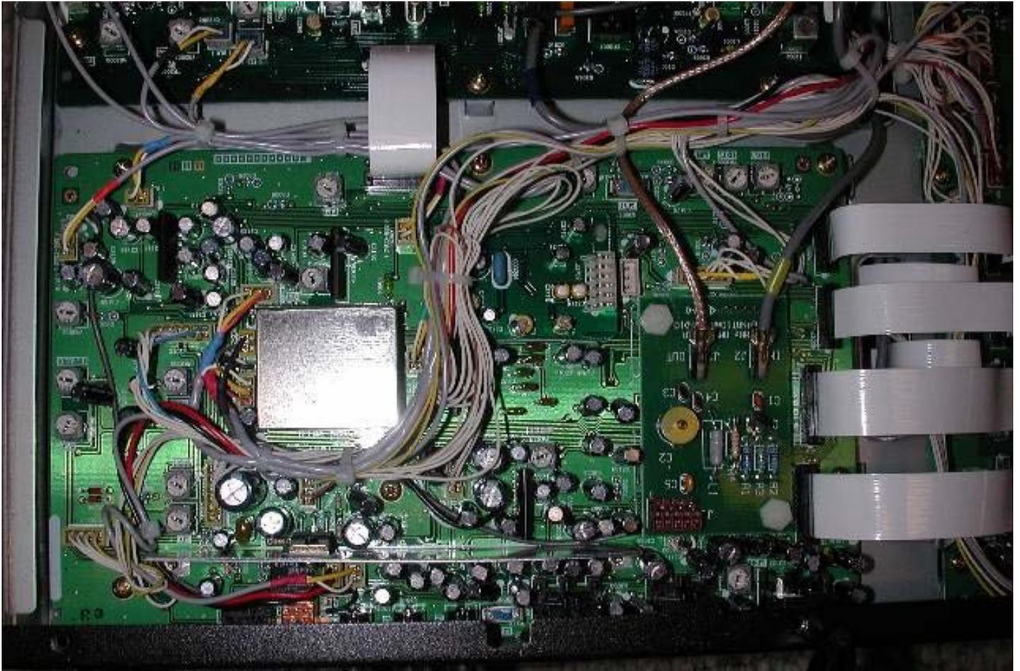
The picture below shows the filters installed. This is the board that will have the rest of the key click mod work. The ribbon cables at the right side are the ones you will need to remove so that you can get at the back of the board. Once you remove the ribbon cables you remove the board mounting screws and flip the board so that the top as we see it here is at the bottom. (See picture following the one below).
