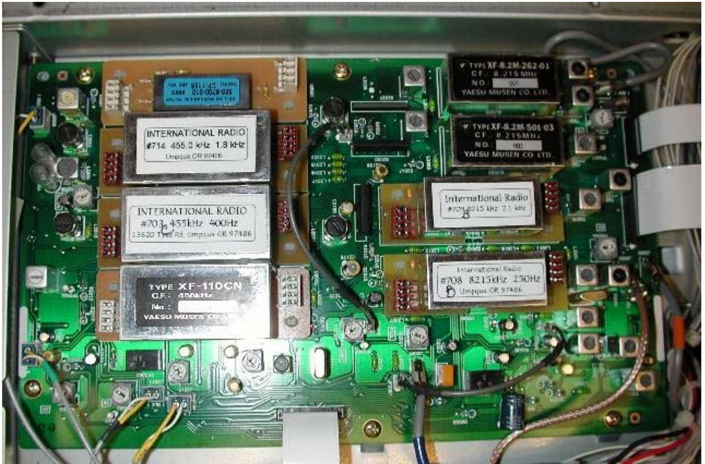
Below is a picture of the 'flipped' board. The top of the unflipped board is now the bottom.. Notice where I put the black (ground) wire from my little perf board. The yellow orange wire is the one that goes from the junction of R1 and C1 in the W8JI URL reference above to the capacitor. Look for the very distinctive trace. The wires wrap around the edge of the board and go to the perf board which will be mounted on the cable bundle to provide easy access to the trimmer pots.
